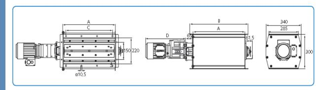
ADS's Rotary Valve, Type STRV-S, has 6 rotor arms with Hard-wearing rubber blades bolted to them. The rotor shaft is directly coupled to a geared motor and attached by a flanged bearing at the opposite end. A tight connection between the rotor and the rotor housing, both made from 3mm thick steel plate, is ensured by the mounting of rubber seals. The units are painted in RAL 5010.
